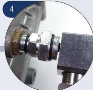
4 Align coupler to coupling fitting
